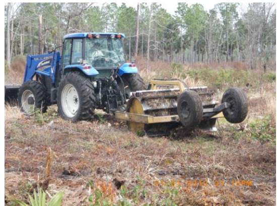
Roller chopping can effectively prepare a site for planting by breaking down hardwoods and debris, but resprouting will often be an issue, photo by Chris Demers.
